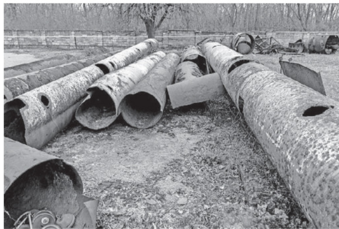
From left: lab workers testing Mykolaiv's water supply; water pipes removed after they were corroded by saltwater; carting bottled water. Denmark adopted Mykolaiv in 2022, and has invested nearly $250 million in the city and the surrounding region. Much of that has gone to repair its fresh water supply, which was destroyed by Russian strikes.
